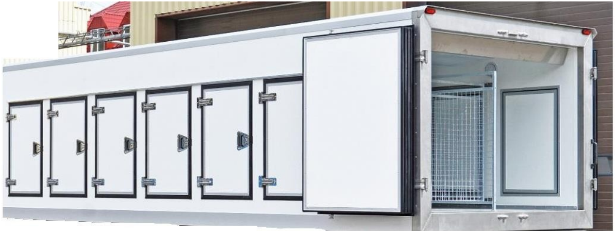
Figure 2.1. Module for separate collection of ground type waste
