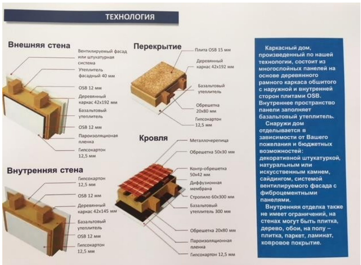
Figure 2. The main elements of the planned production of frame-panel wooden houses
